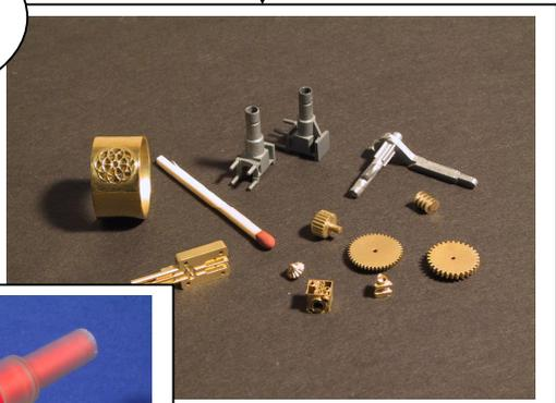
Prototypes for gear, switch, investment cast in metal wax patterns
